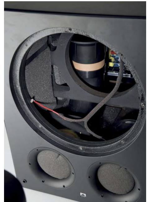
A couple of pictures I snatch from my previous test of 12.17 shows how well the box is, and partly the element in all its shine. Nothing blings right, but look for example, on the constant loss of speaker cables connected. Also note the threads from the contacts to the number pole is fixed in several places in the spider.
